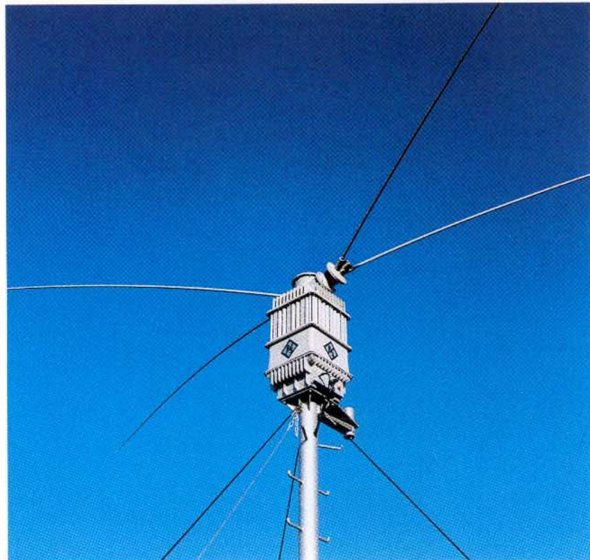
HF Dipole HX002 (2 to 30 MHz) with integrated tuning unit
